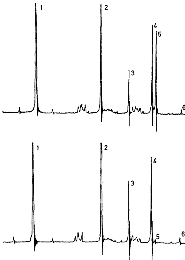
FIGURE. 60MHz N.m.r. spectra: upper trace: Hg(OAc) 2 + DSS in D 2 O 10 min after mixing. Lower trace: same, after 1 h. (1) HOD. (2) MeCO 3 - . (3) MeHgOAc. (4) 'Demethylated' DSS. (5) DSS. (6) 199 Hg satellite of MeHgOAc.
