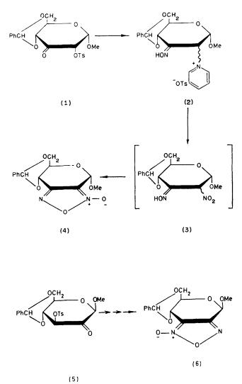
yield 657 mg (58%), m.p. 169–170°,  $[\alpha]_D^{25} + 130^\circ$  (c 1.0, chloroform);  $\lambda_{max}$  (ethanol) 210 ( $\epsilon$  11,000) and 262 nm (8100) (furoxan<sup>4</sup>);  $v_{max}$  (chloroform) 1640 (C=N), 1480-1460 (O-N $\rightarrow$ O), 1390 cm.<sup>-1</sup> (N-O); m/e 306 (M)<sup>+</sup>, 290  $(M - 16)^+$  (diagnostic for N-oxide<sup>5</sup>).
