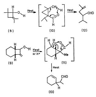
However, the ring contraction of (9) in acidic medium (5% aq.  $H_2SO_4$ ,  $100^\circ$ ) can be followed by n.m.r. which shows the formation of the intermediate (11) which then rearranges to (13) on further heating. As we know that the ring contraction of the cyclobutanol (3) leads to the same product (4), on heating or under acidic conditions, it follows that (10) and (11) can be assumed to be intermediates in the thermal rearrangement.
