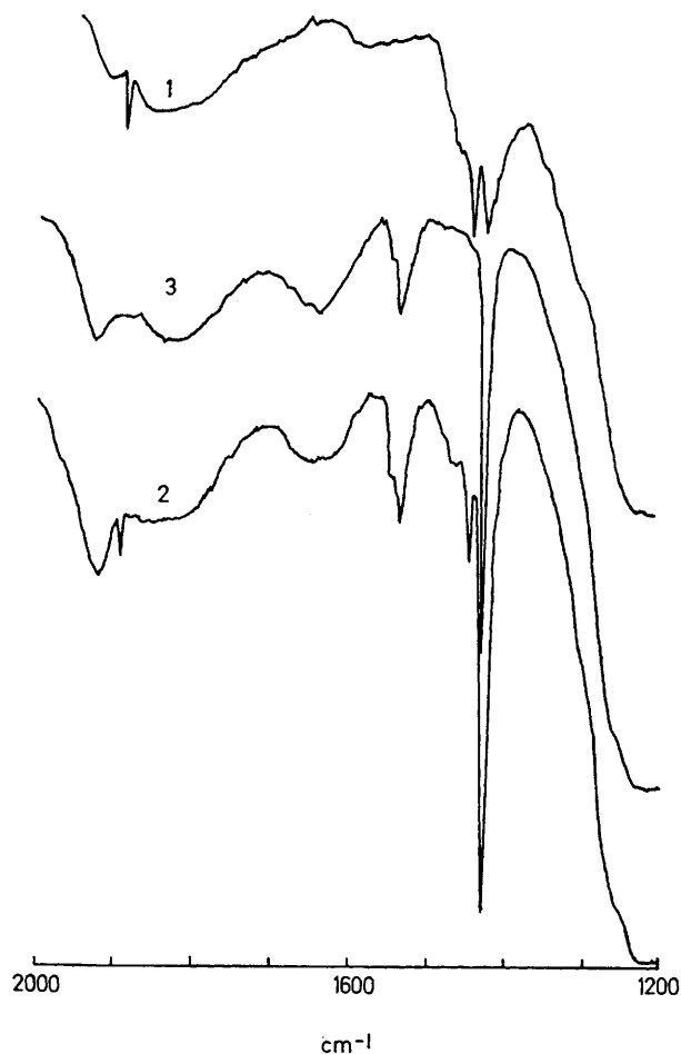
FIGURE. I.r. spectra of copper(I)-ethylene complex in Y zeolites at 25°.
