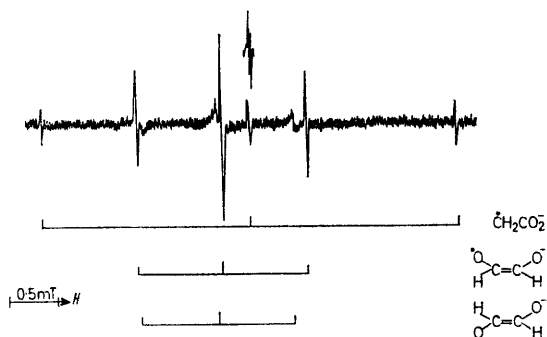
FIGURE. E.s.r. spectra recorded during photolysis of H 2 O 2 (0.16 M) in the presence of ethylene glycol (1.6 M) at pH 9.6 and 3 °C. Modulation amplitude 0.01 mT (insert 0.0063 mT), microwave power 1 mW. Under these conditions lines from \dot{\text{C}}\text{H}_2\text{CHO} are invisible.
