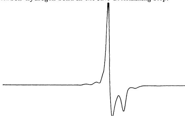
FIGURE 1. The liquid nitrogen temperature e.s.r. spectrum of chromium(V) formed during the chromyl acetate ( 2.5 \times 10^{-3} M) oxidation of ethylbenzene (0.20 M) in acetic anhydride. The centre of the band corresponds to g = 1.971 .
