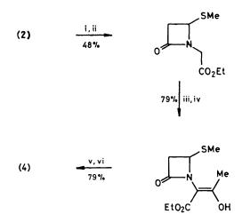
SCHEME. Reagents: i, NaH (1 equiv.), dimethylformamide, 0 °C, 10 min; ii, BrCH<sub>2</sub>CO<sub>2</sub>Et (1·1 equiv.), 0 °C, 1 h; iii, LiN(SiMe<sub>3</sub>)<sub>2</sub> (2 equiv.), tetrahydrofuran, -70 °C, 10 min; iv, MeCOCl (1 equiv.), -70 °C, 1·5 h; v, Cl<sub>2</sub> (1 equiv.), CCl<sub>4</sub>, 0 °C, 5 min; vi, Et<sub>3</sub>N (1 equiv.), tetrahydrofuran, 0 °C, 5 min. Overall yields of each step are given.
