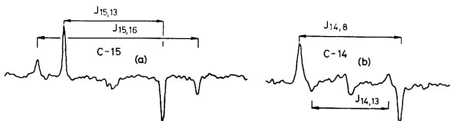
Figure 2. Section of (a) C-15 and (b) C-14 signals from the 100.61 MHz 'INADEQUATE' ^{13}\text{C} n.m.r. spectrum of ( 1 ). Optimization at J = 60 Hz ( J\tau = 1/4 ); satellites due to small ( J_{14,13} 33.2 Hz) and to large ( J_{15,16} 70.0 Hz) coupling constants appear with reduced intensity and in the case of J_{14,13} with opposite sign. 2
