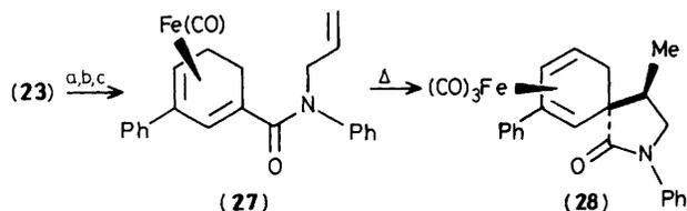
**Scheme 7.** Reagents: a, KOH, MeOH, room temp., 12 h; b, (COCl)<sub>2</sub>, CH<sub>2</sub>Cl<sub>2</sub>, room temp., 3 h; c, pyridine, *N*-allylaniline, C<sub>6</sub>H<sub>6</sub>, 16 h.
