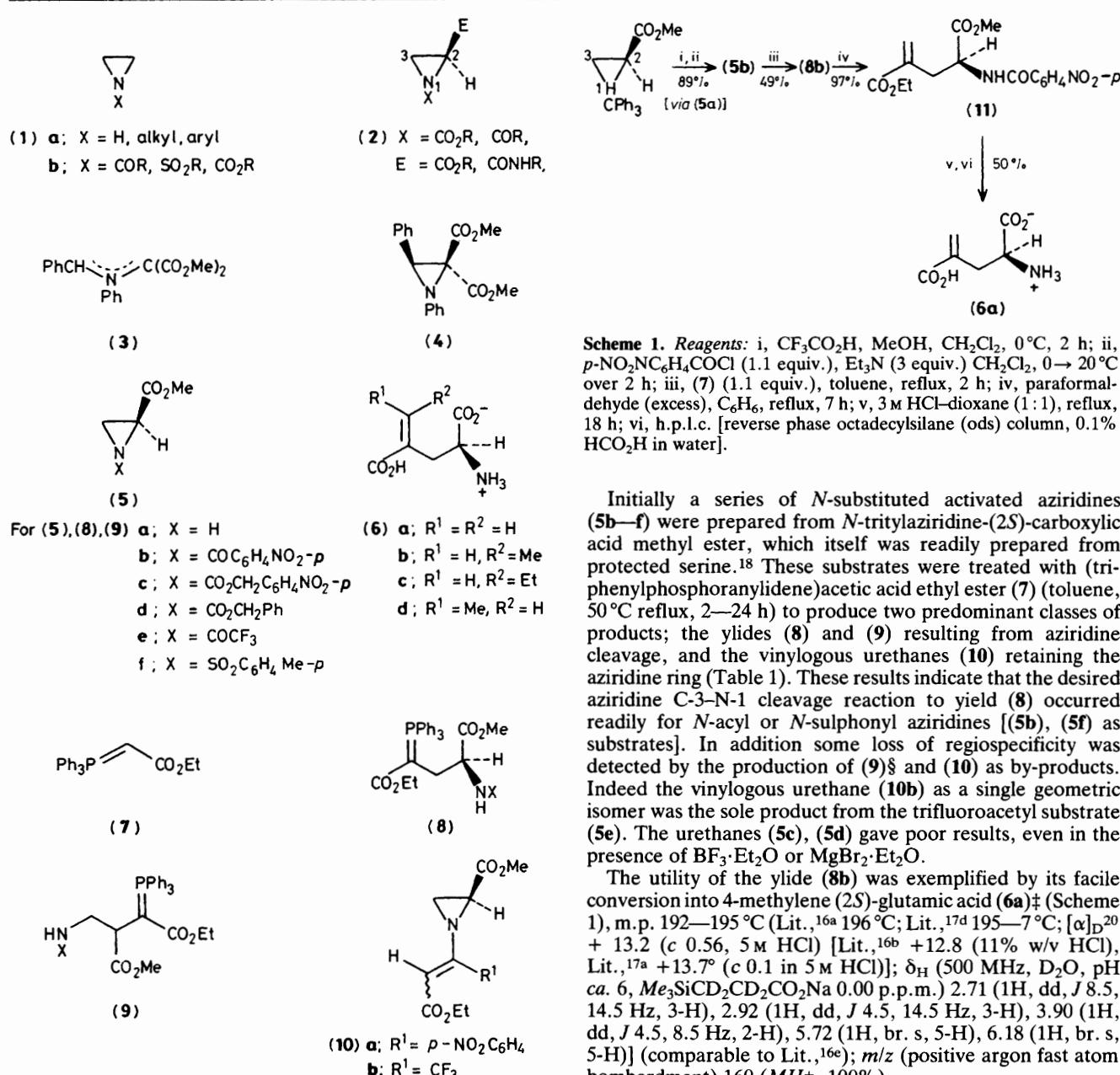
**Scheme 1.** Reagents: i, CF<sub>3</sub>CO<sub>2</sub>H, MeOH, CH<sub>2</sub>Cl<sub>2</sub>, 0°C, 2 h; ii, p-NO<sub>2</sub>C<sub>6</sub>H<sub>4</sub>COCl (1.1 equiv.), Et<sub>3</sub>N (3 equiv.) CH<sub>2</sub>Cl<sub>2</sub>, 0–20°C over 2 h; iii, (7) (1.1 equiv.), toluene, reflux, 2 h; iv, paraformaldehyde (excess), C<sub>6</sub>H<sub>6</sub>, reflux, 7 h; v, 3 M HCl-dioxane (1:1), reflux, 18 h; vi, h.p.l.c. [reverse phase octadecylsilane (ods) column, 0.1% HCO<sub>2</sub>H in water].
