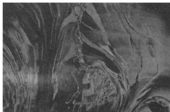
Figure 1. Photomicrograph of bis( N -hexyloxy, 4-decyloxybenzoyloxy-salicylaldehyde)nickel(II) in its nematic phase at 155^{\circ}\text{C} viewed between crossed polars.
