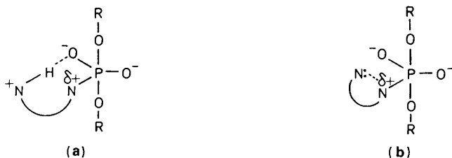
Figure 1. Proposed mechanisms for the catalysis by (a) the monocations and (b) the neutral diamines. R represents the nitrophenyl residue, and the methyl groups on the nitrogen atoms are omitted for clarity.
