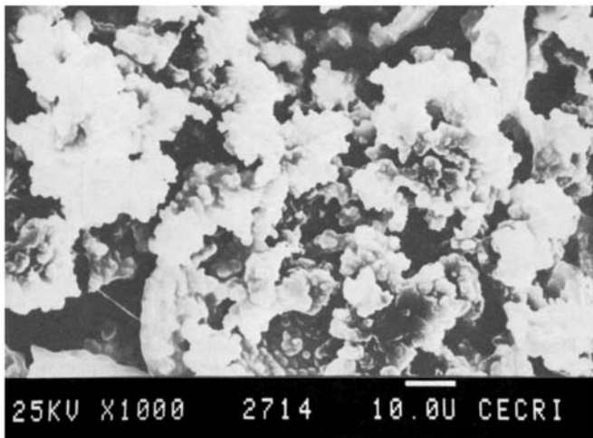
Figure 2. Scanning electron micrograph of the polymer, showing at least one superstructure.
