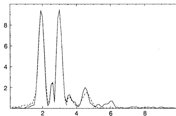
**Figure 2.** Observed (—) and calculated (----) Fourier transform (quasi-radial distribution function) of  $k^3$ -weighted Ir  $L_{III}$ -edge EXAFS spectrum for (4) in 200 mmol  $\text{dm}^{-3}$  methanol solution.
