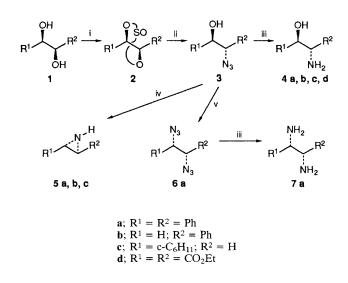
Scheme 1 Reagents and conditions: i, SOCl<sub>2</sub>, CCl<sub>4</sub>; ii, LiN<sub>3</sub>, DMF, 120 °C; iii, H<sub>2</sub>/Pd·C or LiAlH<sub>4</sub>, THF, heat; iv, PPh<sub>3</sub>, THF, heat; v, a, MsCl-Py; b, LiN<sub>3</sub>, DMF, 120 °C
