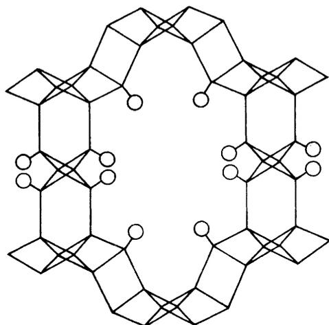
**Fig. 1** View of the 20-ring channel showing the connectivity of the tetrahedral sites and location of the oxygen atoms (open circles) protruding into the channels
