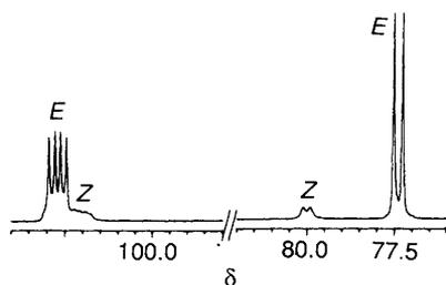
**Fig. 1**  $^{15}\text{N}$  NMR spectrum of  $\text{Boc-}^{15}\text{NH-}^{13}\text{CH}_2\text{-}^{13}\text{CO-}^{15}\text{NH}_2$  **4a** in  $\text{CDCl}_3$  (0.5 mol  $\text{dm}^{-3}$ ) at 50.7 MHz (276 K)
