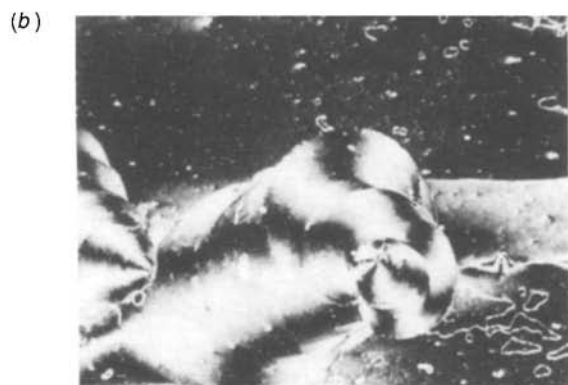
Fig. 1 Photographs of the spiral texture using (a) polyimide treated by rubbed technique and (b) octadecyltriethoxysilane as the opposite substrate. The photographs were taken between cross polarisers.
