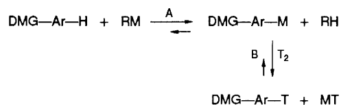
Scheme 1 Metallation/reduction of aryl compounds (DMG = ortho -directed metallation group)
