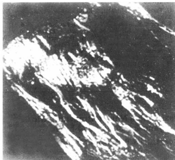
Fig. 2 Liquid crystalline compound 6 (bright area), in cross-polarised transmitted light, on cooling to room temperature
