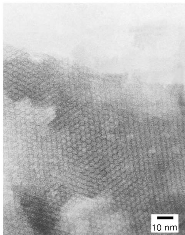
Fig. 3 Transmission electron micrograph of silicate-organic complex. This micrograph was obtained on a JEOL JEM-200CX at an accelerating voltage of 200 kV.
