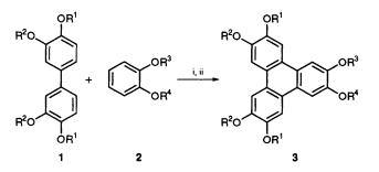
Scheme 2 Reagents: i, FeCl<sub>3</sub>/CH<sub>2</sub>Cl<sub>2</sub>, ii, MeOH
