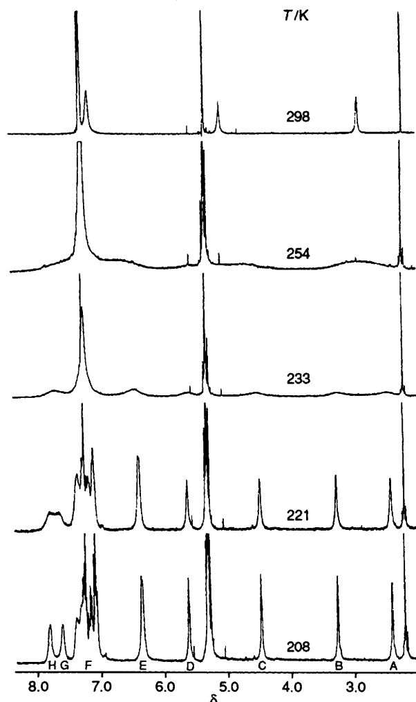
Fig. 2 360.13 MHz ^1\text{H} NMR spectra recorded over a range of temperatures. The coalescence of signals C and D at 254 K gives \Delta G^\ddagger 47.43 kJ mol -1 for the ligand 'swivel' process.
