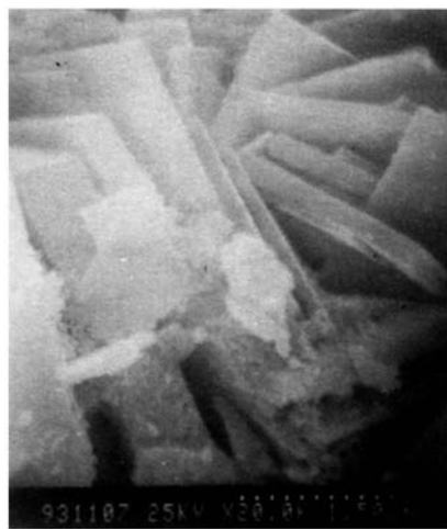
Fig. 2 Scanning electron micrographs of \text{AlPO}_4\text{-17}
