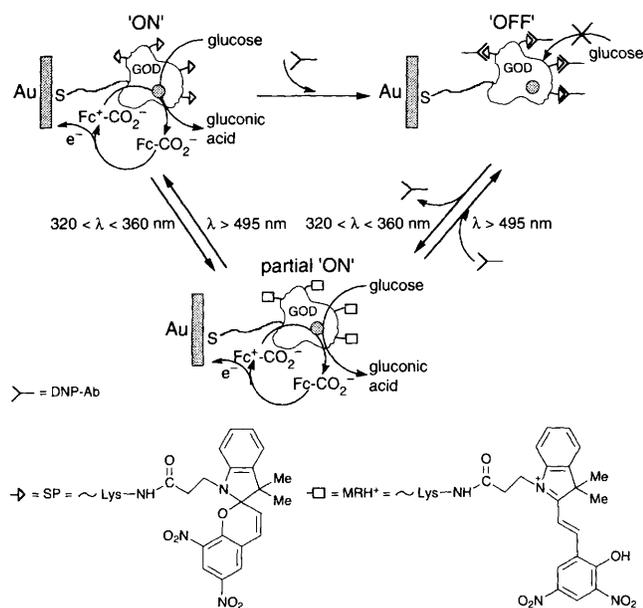
Fig. 2 Schematic operation of the biphasic switch of a dinitrospiropyran-GOD monolayer electrode in the presence or absence of the DNP-Ab
