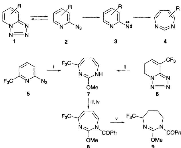
**Scheme 1** Reagents and conditions: i, *hν*, dioxane–methanol (3 : 1), 25 °C, 80 min, 92%; ii, as in (i), 47%, ca. 5% of 2-amino-3-trifluoromethylpyridine also formed (GC–MS); iii, BuLi, THF, –80 °C; iv, PhCOCl, –80 °C, 87%; v, H<sub>2</sub>/Pd, MeOH, 25 °C, 14 h, 87%.
