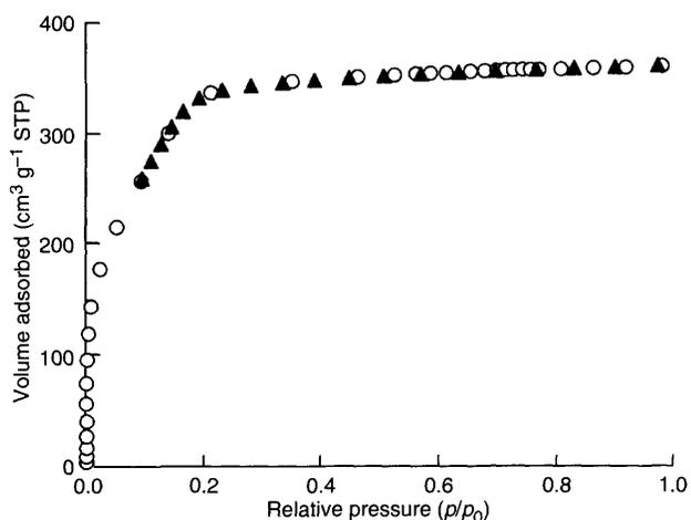
Fig. 2 Nitrogen adsorption–desorption isotherms for the calcined silica–C<sub>16</sub>TAC composite. Before the measurement the sample was heated for 3 h at 393 K. The isotherms were measured at 77 K.
