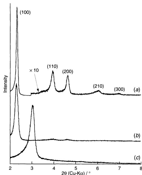
**Fig. 1** X-Ray diffraction patterns of (a) the silica-C<sub>16</sub>TAC composite film (TMOS:C<sub>16</sub>TAC molar ratio = 4:1), (b) the silica-C<sub>16</sub>TAC composite and (c) calcined (b)
