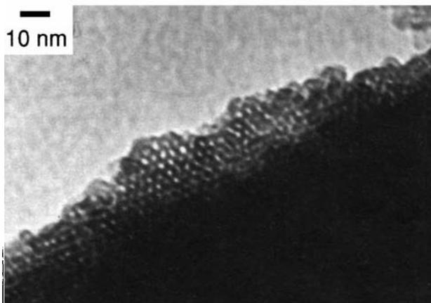
Fig. 3 Transmission electron micrograph of the calcined silica–C<sub>16</sub>TAC composite
