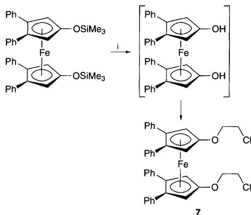
**Scheme 2** Synthesis of the ferrocenyl alkyl ether **7** via intermediate dihydroxyferrocene. *Reagents and conditions:* i, Na<sub>2</sub>CO<sub>3</sub>, DMF, 80 °C, + ClC<sub>2</sub>H<sub>4</sub>(OSO<sub>2</sub>C<sub>6</sub>H<sub>4</sub>Me).
