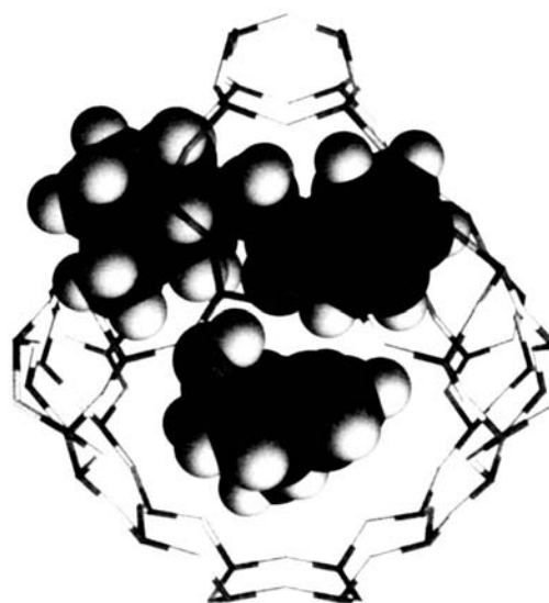
Fig. 1 Molecular model diagram of ephedrine and ketone 1 within the supercage of X or Y zeolite. Guest structures have been minimized but the guest–host assembly has not. The figure shows that both the ephedrine and ketone can fit within zeolite cages.
