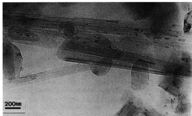
Fig. 3 TEM micrograph of rhodium-filled nanotubes after removal of the externally located rhodium particles by treatment with a reverse micellar solution
