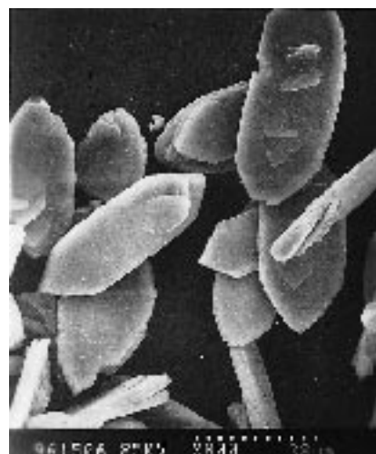
Fig. 2. Scanning electron micrograph of as-synthesized penkviksite
