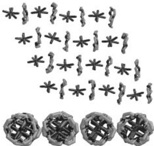
Fig. 2 The asymmetric unit of [\text{UO}_2\text{Cl}_2(\text{H}_2\text{O})_3]_{16}(\text{15-crown-5})_{16} 2 comprising four parallel, helical columns of alternating [\text{UO}_2\text{Cl}_2(\text{H}_2\text{O})_3] and 15-crown-5 (end and side views)
