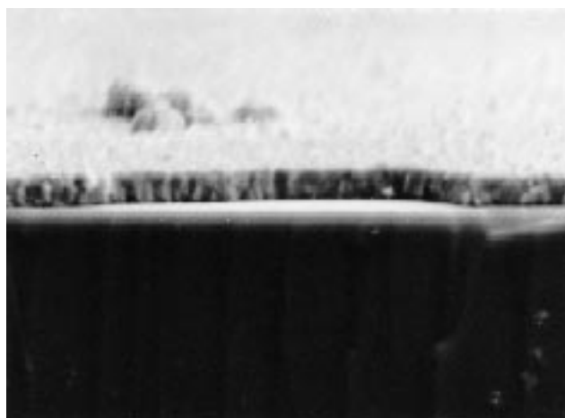
Fig. 1 Typical thin film of CdSe on glass from [\text{Cd}\{\text{Se}_2\text{CNMe}(\text{C}_6\text{H}_{13})_2\}_2] , T_{\text{source}} = 250^\circ\text{C} , T_{\text{growth}} = 450^\circ\text{C} , 2 h growth run; bar is 10 \mu\text{m}
