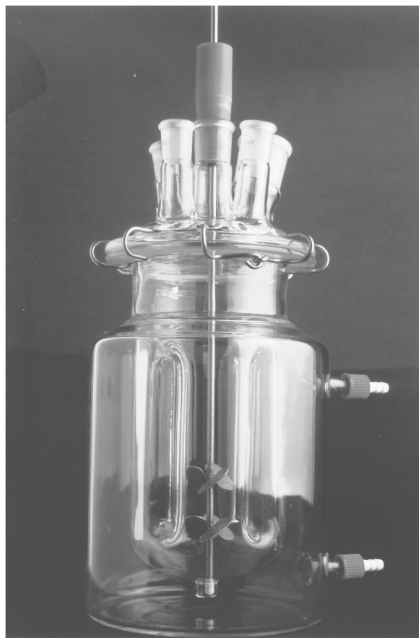
Fig. 10 Suspension polymerisation reactor, internal volume 1 l, used in the author's laboratory.
