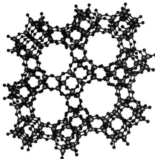
Fig. 3 A perspective view of the framework structure of ITQ-9 down [001], showing the nearly circular one-dimensional 10MR pores (average free diameter \cong 5.7 Å). Large spheres represent tetrahedral Si, while small spheres are two-coordinated O.
