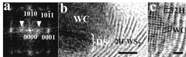
Fig. 3 (a) Calculated ED pattern, obtained from a FFT of the indicated region in Fig. 2(b) corresponding to the WC/2H-WS 2 interface. The 0002 reflections of the sulfide are arranged along [0001] with respect to the carbide. (b) HRTEM micrograph showing the WC/2H-WS 2 interface. A distorted region (DS) is visible in the carbide microstructure (scale bar \approx 35 Å). (c) Enlargement of the WC/2H-WS 2 interface showing intergrowth between two layers of the distorted carbide structure (WC) and one layer of the sulfide (2H; scale bar \approx 10 Å).
