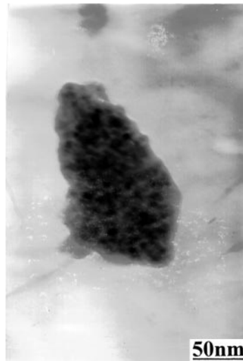
Fig. 4 TEM image of a ZnS-PAM nanocomposite prepared by the in situ simultaneous polymerization-hydrolysis technique (SPH) at 140 °C for 12 h.
