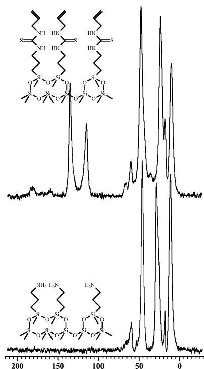
Fig. 2 ^{13}\text{C} CP-MAS NMR spectra for the mesoporous materials functionalized with aminopropyl (MCM-41NH 2 ) and 1-allyl-3-propylthiourea (MCM-41ATU) groups. Chemical shifts are in ppm with respect to TMS standard.
