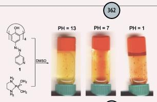
A stable metal coordination polymer gel based on a calix[4]arene and its 'uptake' of non-ionic organic molecules from the aqueous phase
