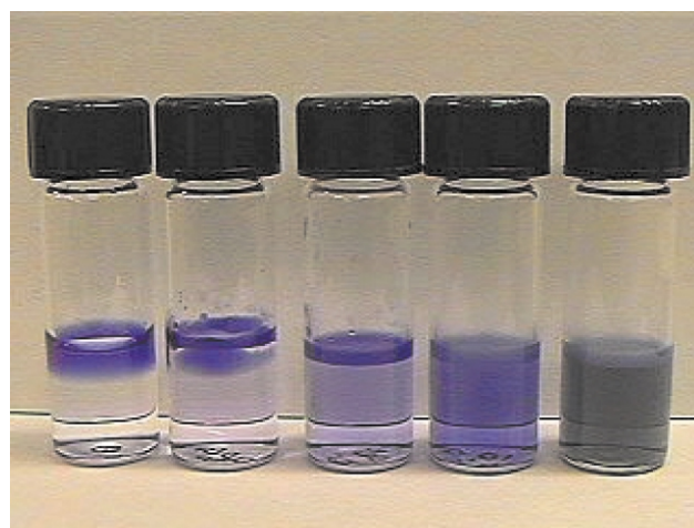
Fig. 2 Extraction of bromophenol blue into HFE by FNAD. Concentrations of FNAD from left to right are 0, 0.015, 0.15, 1.5, and 15 mM.
