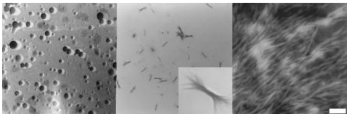
Fig. 1 Transmission electron micrograph of a dispersion of G3OPV in water (pH = 1, picture left, bar represents 400 nm). Transmission electron micrograph of a dispersion of G3OPV in decanol (picture in the middle; bar represent 5 \mu\text{m} ; inset: bar represent 500 nm). Tapping mode atomic force micrograph (picture right; height scale is 22 nm; bar represents 120 nm).
