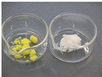
Fig. 1 Photograph of the resin with (left) or without (right) the Mo complex 1 attached. The success of the labelling can be visually verified by the yellow colour of the resin.
