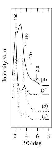
XRD patterns of: (a) as-synthesized HMA; (b) calcined HMA; (c) as-synthesized FeHMA and (d) calcined FeHMA.
