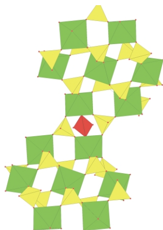
Fig. 2 A representation of two building units of ScSPO, showing the way they are attached. In the structure, each building unit is attached to six others in this way. The colour scheme is the same as for Fig. 1.
