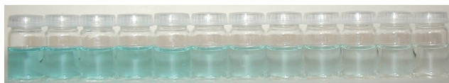
Fig. 2 H 2 O:ACN 80:20, from left to right [CN - ] = 0, 1, 3, 5, 8, 11, 14, 18, 22, 26, 30 and 40 × 10 -5 M, in presence of TRIS 0.01 M after 18 minutes of reaction, [L 1 ] = 1.00 × 10 -5 M.
