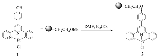
Scheme 1 Synthesis of water soluble polymer supported cyclometalated platinum(II) complex.
