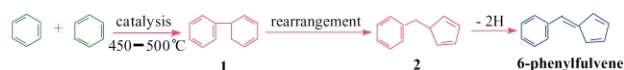
Fig. 1 The mechanism for thermic rearrangement and dimerization of benzene catalyzed by GaP nanocrystals at 450–500 °C.
