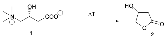
Scheme 1 Solvents and conditions. Off-line: DMSO or DMF, 150 °C, 2 h. On-line: CH 3 NO 2 , GC injection port at 200 °C.
