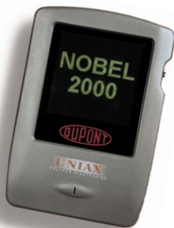
A display built using polymer LEDs made at UNIAX (now DuPont Displays), permission granted by A. J. Heeger
