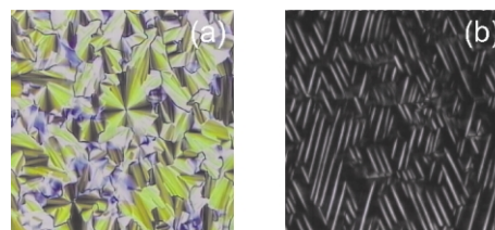
Fig. 1 Polarized optical photomicrographs observed in the columnar phase of the polycatenar compound (a) between normal glass plates at 90 °C, showing a focal-conic texture and (b) between polyimide-coated glass plates at 75 °C, showing a characteristic structure.
